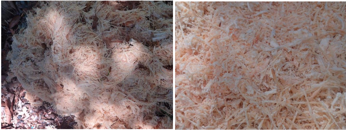
Figure 6: The mixture of fibre and pith collected by means of traditional beating method with mostly largest fibre pieces (left), and grinding method with fibrous pulp observed (right).
