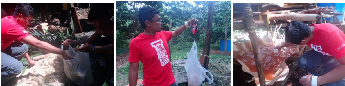
Figure 8: Mr Razi collected the fibrous mash into a plastic bag for weighing (left); Mr Razi weighed on the sago bark (centre); Mr Razi collected sieved water as sample to bring back for further analysis (right).
