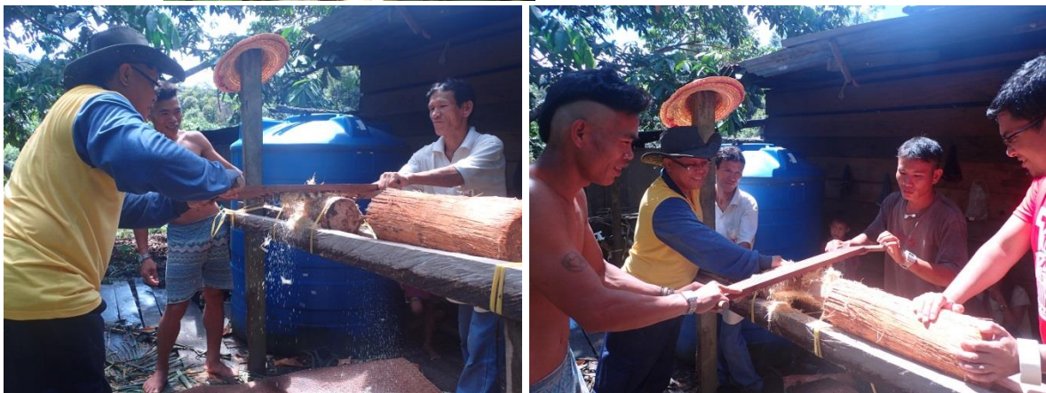
Figure 5: Mr Asai (headman of Lg Si'ang) and a local used a small hoe made from tree stems in rasping the pith (top); Mr Peter and Mr Razi with the locals tried the new rasping instrument using a board with nails in it, on the sago trunk which has been removed its bark (bottom).
